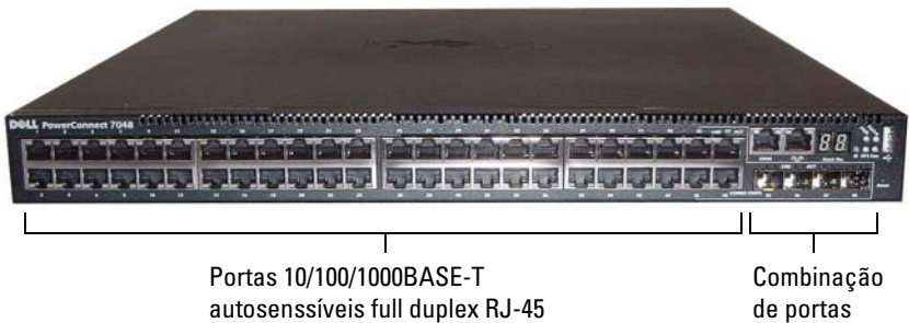
Figura 1-4. PowerConnect 7048 com 48 portas 10/100/1000BASE-T
