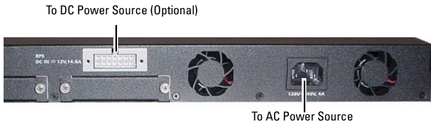
Figure 1-15. AC and DC Power Connection to Switch
